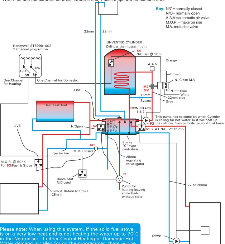
With time and temperature controls. Group 3 and 4 boilers operate on demand only.
